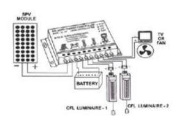
**Technical Description** for solar small home light Lamp : CFL 9 watt/ LED fixture Battery : 12 V, 40/50 / 75 Ah Tubular
